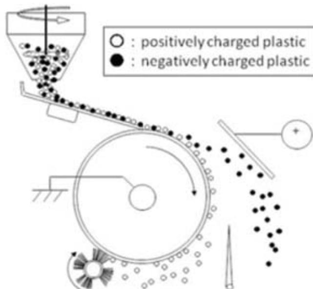
Principle of electrostatic separation<sup>5</sup>
