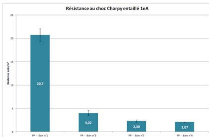
Result of Charpy test sample reactions to impact, taken from four batches
